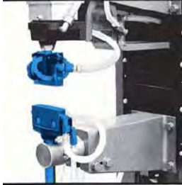
Bar electrode holder water-cooled
